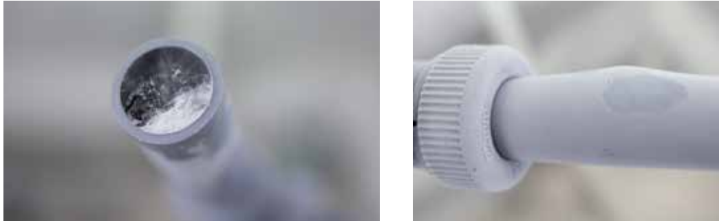
The frozen pipe dilates without breaking, avoiding water leakage in installations exposed to low temperatures.
